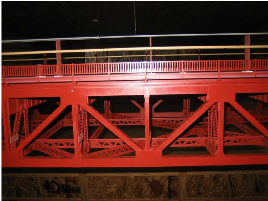
Adding to the existing railing and with above deck winglets (Test number W3)
